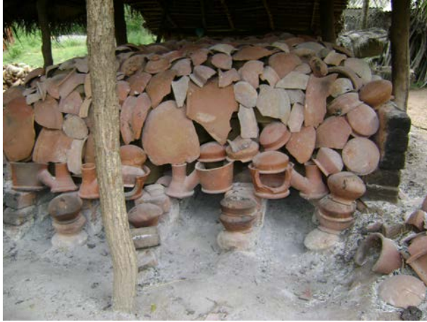
Figure 3.52: Covered with “Kabal” (Damaged pots)
