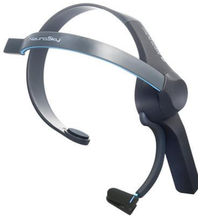
Figure 3.2: NeuroSky mindwave mobile with single dry electrode [38]
