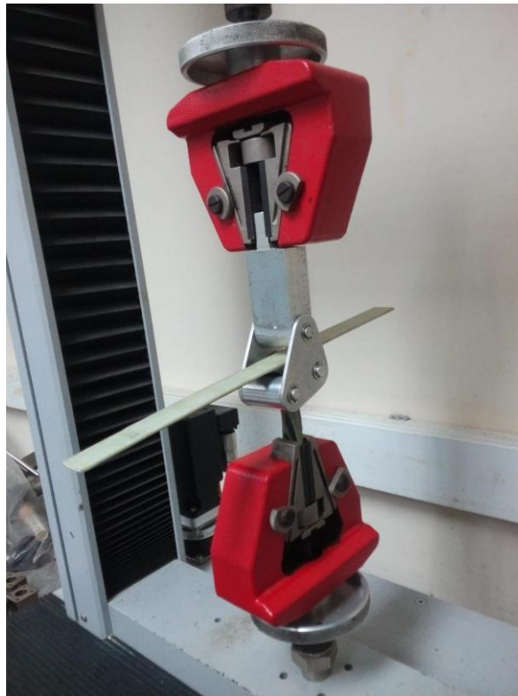
Figure 10: Experimental setup for floating roller peel test
