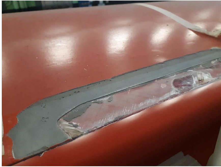
Figure 4: Removed tab of a de-bonded tab
