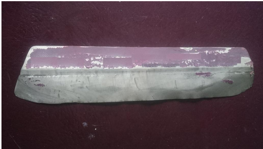
Figure 23: Peeled off tab piece
