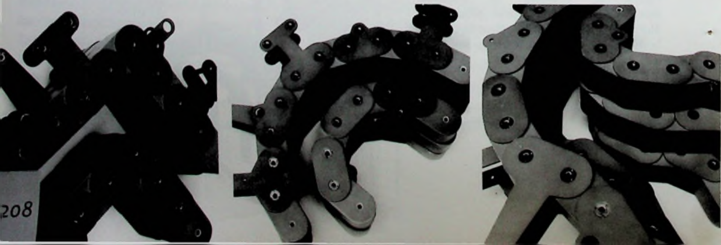
Figure 05: A quarter-scale model of the Shok-Mod 05S, digital/mechanical formwork. Right-angle configuration (right), radius/curvilinear (middle), and free-form/open. Models and photographs by the author.
