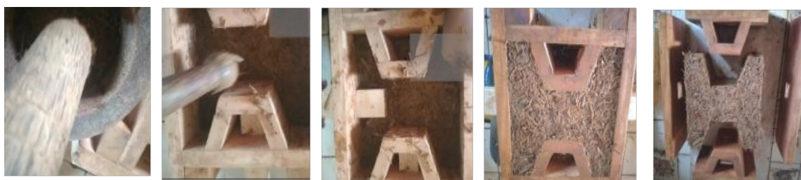
Figure 5: Manufacturing process with manual molding technique
