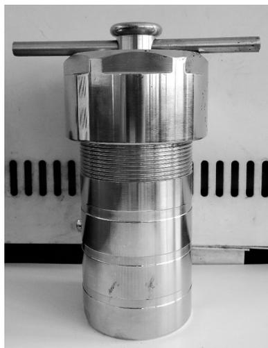
Fig. 6.2: Hydrothermal autoclave synthesis reactor used for experimentation
