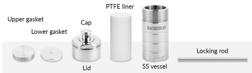
Fig. 6.3: Structural parts of hydrothermal synthesis reactor
